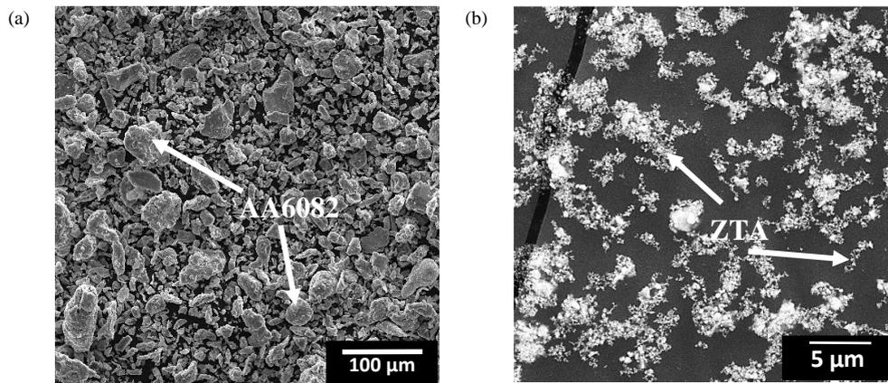
Fig. 1. Scanning electron micrograph of (a) AA6082 powder and (b) ZTA powder
