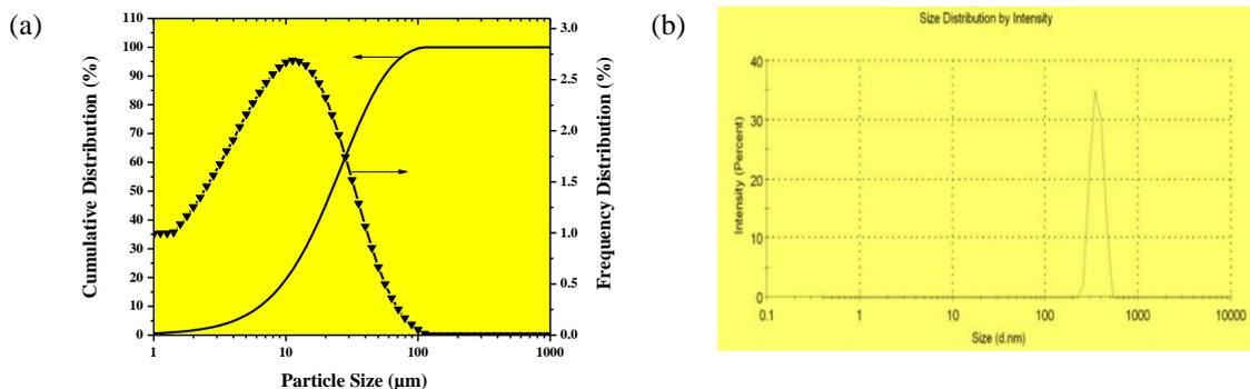
Fig. 3. Particle size distribution of (a) AA6082 and (b) ZTA
