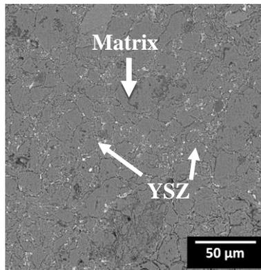
Fig. 5. Microstructure of sintered ZTA composites with 9 wt.% ZTA pressed at 500 MPa and sintered at 560°C for 60 min.
