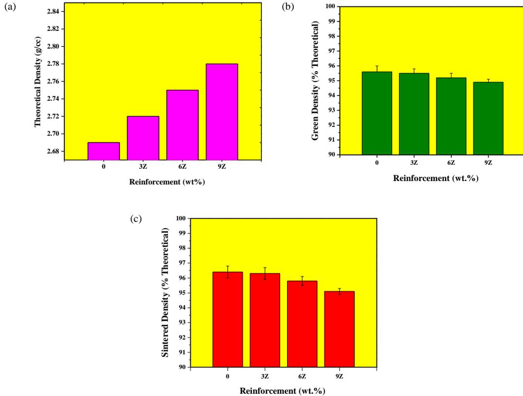
Fig. 4. (a) Theoretical Densities (b) Green Densities (c) Sintered Densities of AA6082 and its composites
