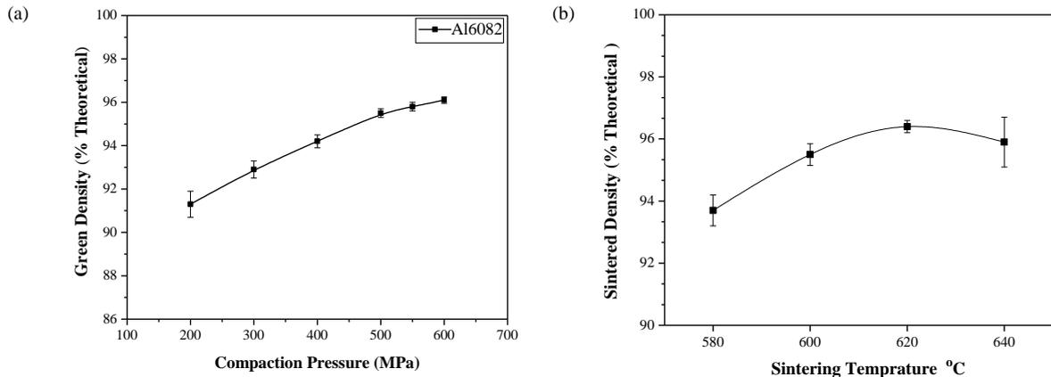
Fig. 2. (a) Compressibility curves of AA6082 alloy and (b) Sinter density versus sintering temperature of AA6082 alloy
