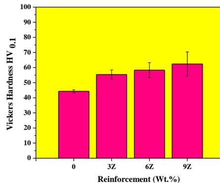
Fig. 3. Effect of ZTA Addition on the Hardness
