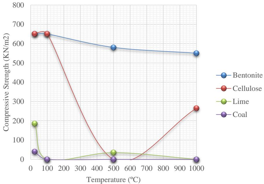
Fig. 5. Effect of temperature on the compressive strength of iron concentrate briquettes
