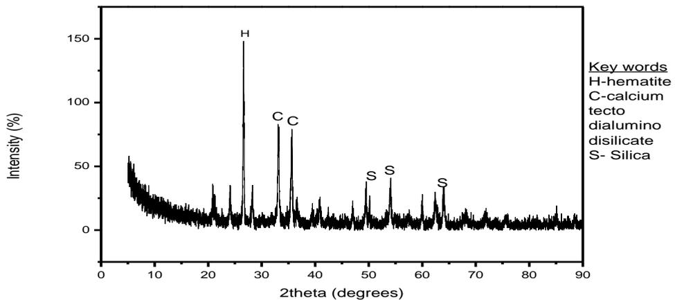
Fig. 2. XRD pattern of the fluorspar tailings
