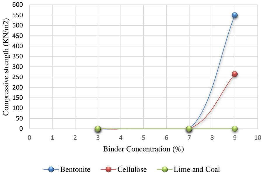
Fig. 4. Effect of binder concentration on compressive strength on iron briquettes
