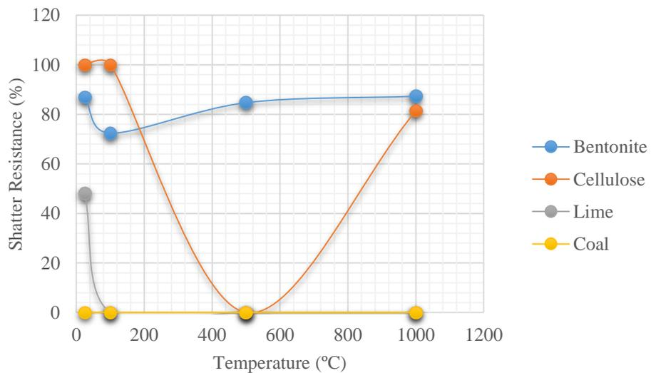
Fig. 6. Effect of temperature on the shatter resistance of iron briquettes
