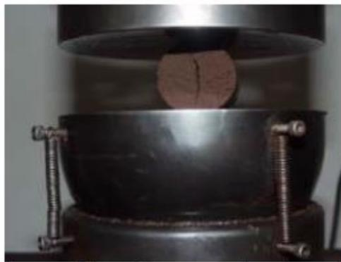
Figure 1: Compressive strength testing machine
