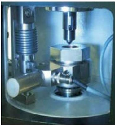
Fig. 1(a) Four ball testing assembly
