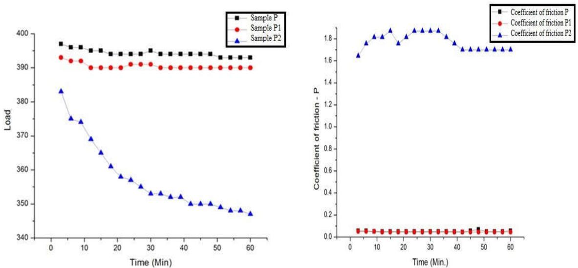
Graph 2. Petrol engine oil sample (a) Load vs time;
