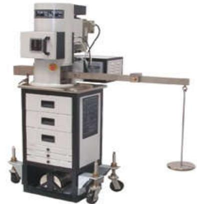
Fig. 1(b) Four ball tester
