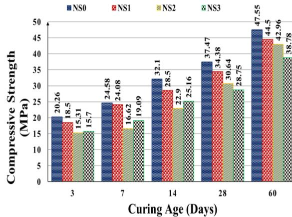
Fig. 1. Compressive strength of PPC cement mortar
