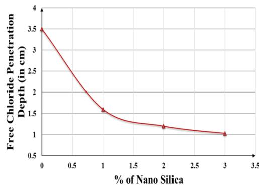
Fig. 2. Chloride penetration test of PPC cement mortar
