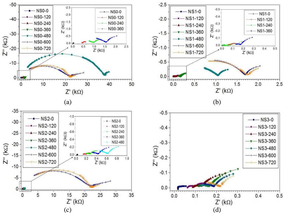
Fig. 3. Impedance spectra for different % of nano-SiO<sub>2</sub> in PPC cement paste for (a) 0, (b) 1, (c) 2 and (d) 3
