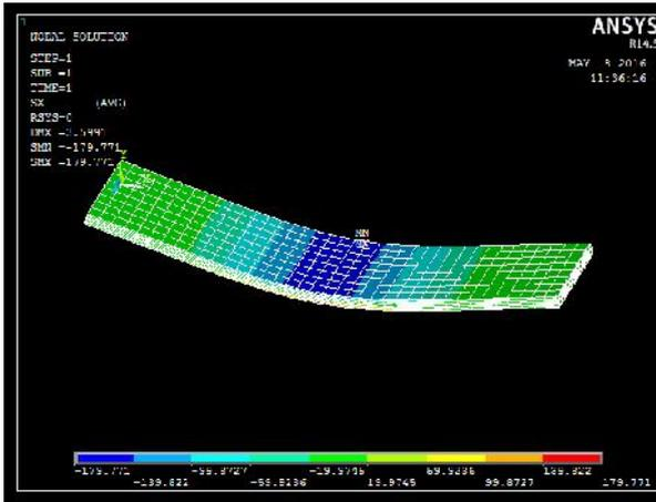
Fig. 12 nodal solution for bending stress for X component (sample 3)
