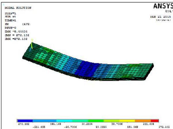
Fig. 10 nodal solution for bending stress for X component (sample1)
