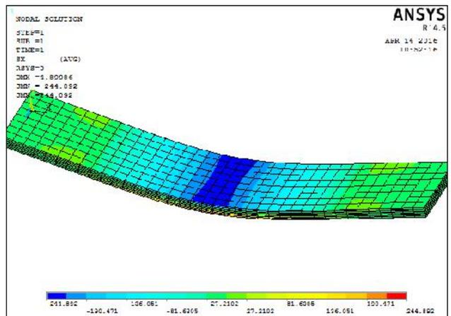
Fig. 11 nodal solution for bending stress for X component( sample2)
