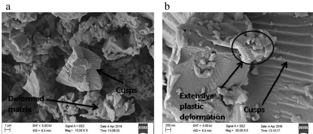
Fig. 8. FE- SEM image of fracture surface of unfilled GFRP composite (a) deformation behaviour of matrix at 1µm; (b) Cusps at 200 nm.
