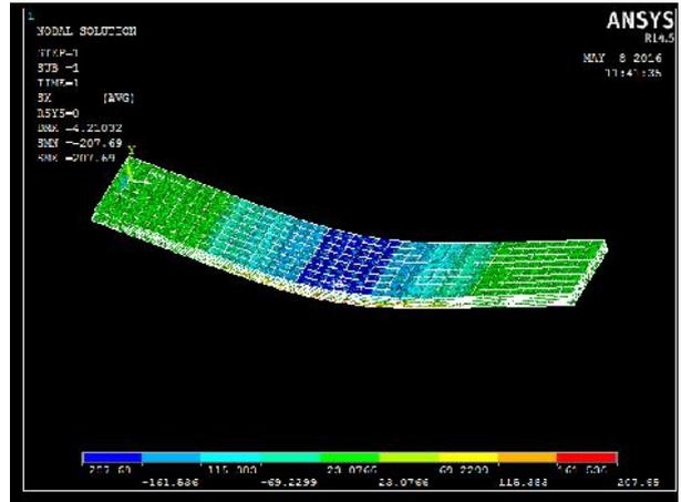
Fig. 13 nodal solution for bending stress for X component (sample 4)
