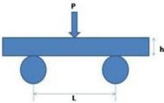
Fig.2 Three point bend test
