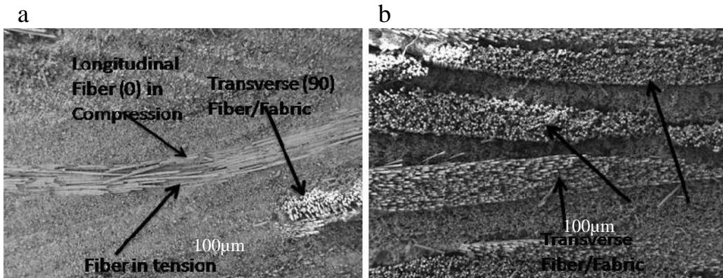
Fig. 5 FE- SEM image of fracture surface of unfilled GFRP composite at 100 μm showing (a) longitudinal fiber; (b) transverse fiber
