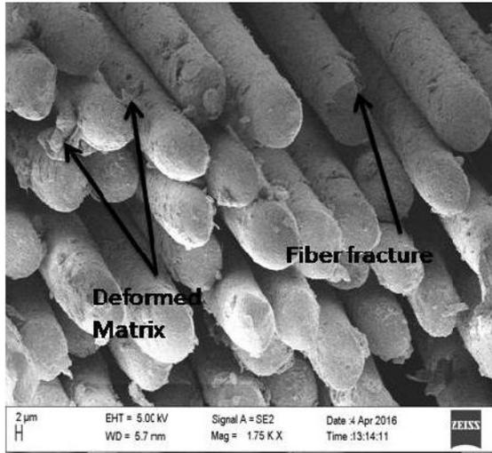
Fig. 9. FE- SEM image of fracture surface of unfilled GFRP composite showing arranged fiber at 2 μm.
