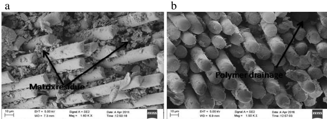
Fig. 7. FE- SEM image of fracture surface of unfilled GFRP composite (a) matrix residue; (b) thin layer of matrix covering the glass fiber
