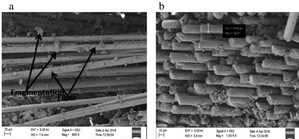
Fig. 6. FE- SEM image of fracture surface of unfilled GFRP composite showing (a) fabric fragmentation; (b) well arranged fiber
