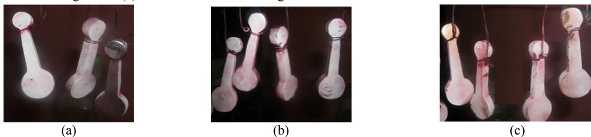
Figure 5: Liquid penetrant inspection of A356 aluminum alloy Connecting rod castings made in (a) 100% Sand mould (b)100% GBF Slag mould (c) Mixture of 50% GBF Slag+50% Sand mould.
