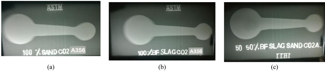
Figure 9: Radiography testing images of A356 alloy Connecting rods made in: (a) 100% Sand mould (b)100% GBF Slag mould (c) Mixture of 50% GBF Slag+50% Sand mould
