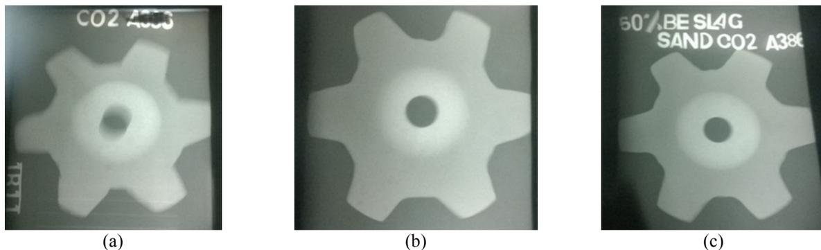
Figure 8: Radiography testing images of A356 alloy Gear wheel made in: (a) 100% Sand mould (b) 100% GBF Slag mould (c) Mixture of 50% GBF Slag+50% Sand mould
