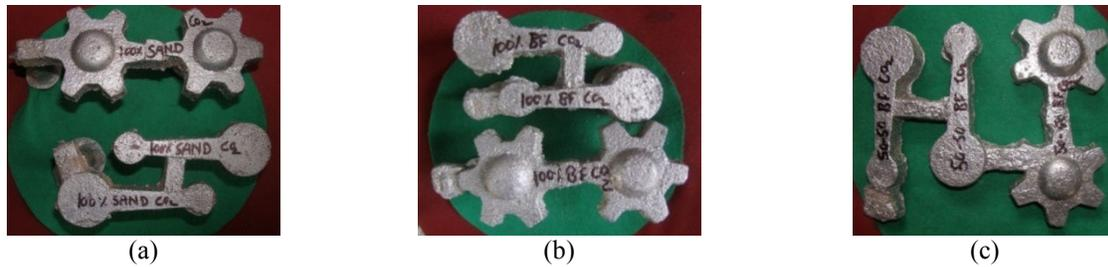
Figure 1: A356 Aluminum alloy castings before machining casted in: (a) 100% Sand mould (b) 100% GBF Slag mould (c) Mixture of 50%GBF Slag + 50% Sand mould
