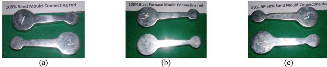
Figure 3: Visually inspected A356 alloy Connecting rod castings made in: (a) 100% Sand mould (b)100% GBF Slag mould (c) Mixture of 50% GBF Slag+50% Sand mould
