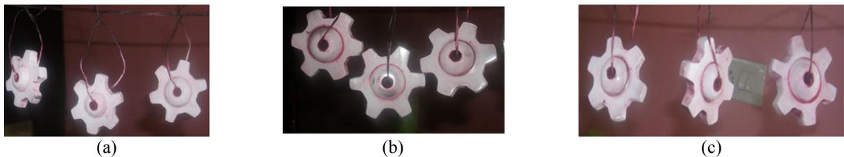
Figure 4: Liquid penetrant inspection of A356 aluminum alloy Gear wheel castings made in (a) 100% Sand mould (b)100% GBF Slag mould (c) Mixture of 50% GBF Slag+50% Sand mould.
