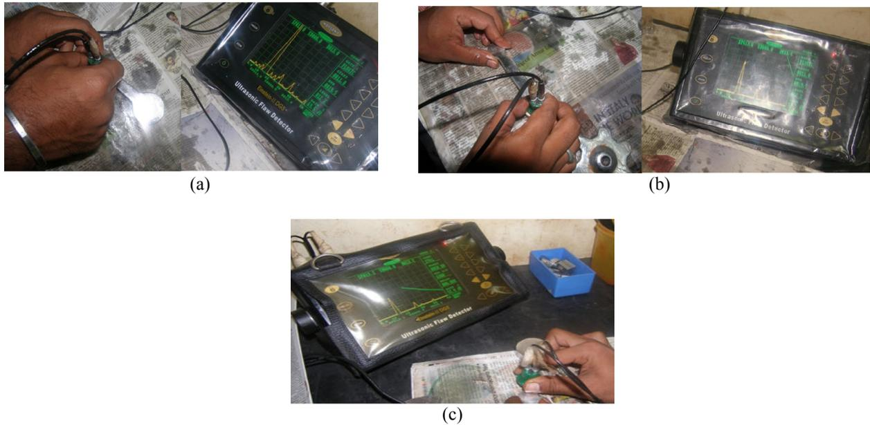
Figure 7: ultrasonic Inspection of connecting rod aluminum alloy A356 castings poured in (a) 100% Sand Mould (b) 100% GBF Slag mould (c) Mixture of 50% GBF Slag+50% Sand mould.
