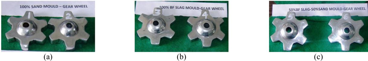
Figure 2: Visually inspected A356 alloy Gear wheel castings made in: (a) 100% Sand mould (b)100% GBF Slag mould (c) Mixture of 50% GBF Slag+50% Sand mould.
