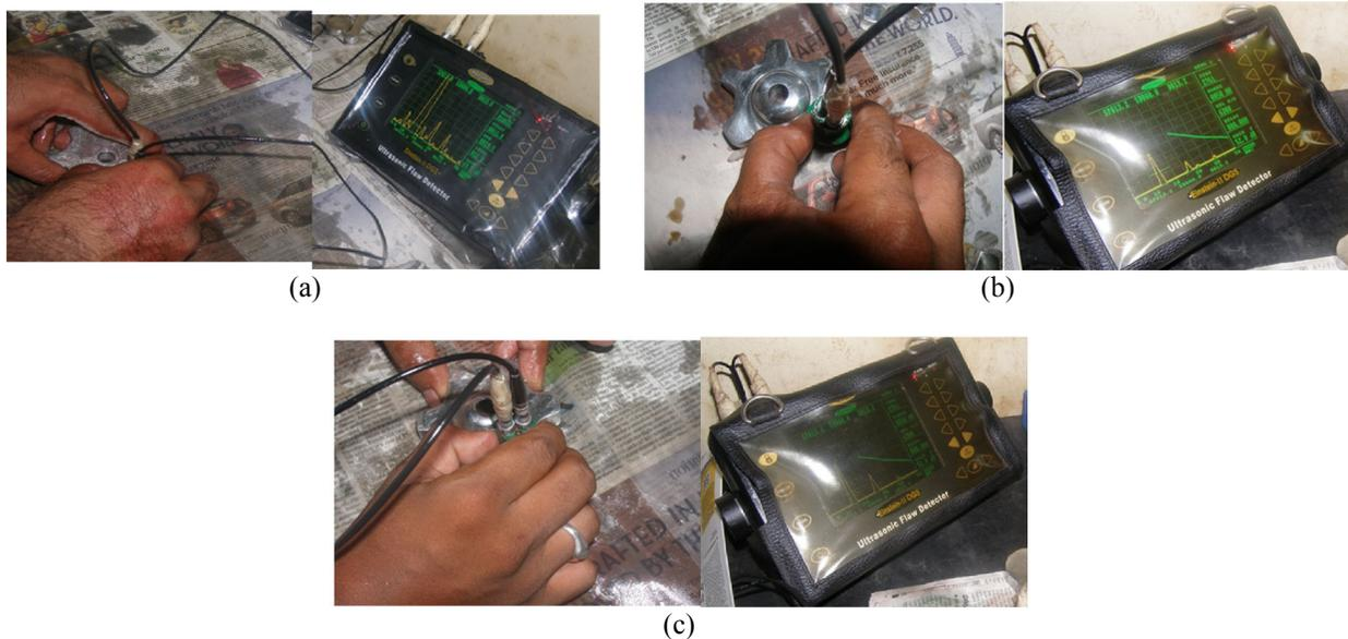
Figure 6: ultrasonic Inspection testing of Gear wheel aluminum alloy A356 castings poured in (a) 100% Sand Mould (b) 100% BF Slag Mould (c) Mixture of 50% GBF Slag+50% Sand mould.
