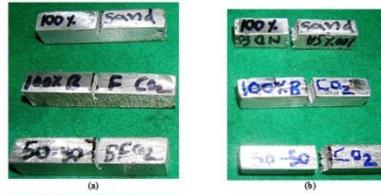
Figure 5: Charpy impact specimens: (a) before testing (b) after testing
