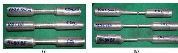
Figure 3: A 356 alloy Tensile specimens: (a) before testing (b) after testing.
