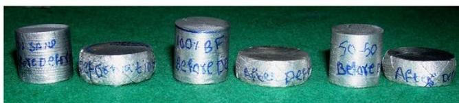
Figure 4: Cylindrical samples with aspect ratio = 1.0 showing bulge profiles before and after deformation under compression
