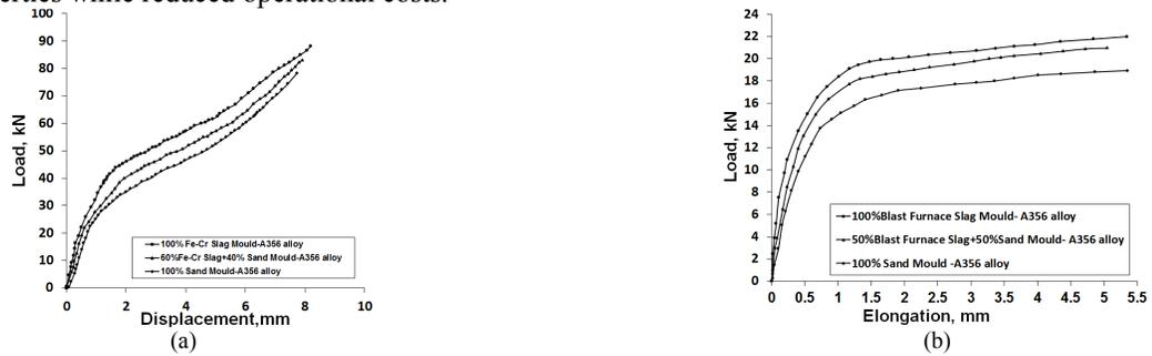
Figure 9: (a) Load- displacement curves under compression testing for aspect ratio (H/D) =1.0 and (b) Load- elongation curves under tensile testing.
