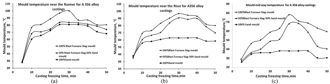
Figure 6: Variation in mould temperatures at various locations during freezing of A356 alloy castings for Sand, GBF slag and mixture of these two moulds: (a) near the Runner (b) near the Riser, and (c) Midway of the mould.
