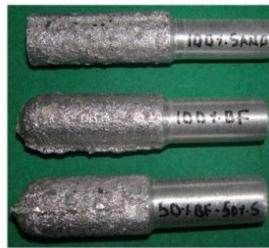
Figure 1: A 356 alloy finished cylindrical castings before and after machining
