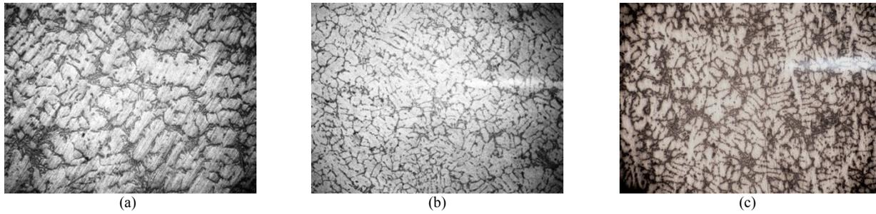
Figure 7: Microstructure of A356 aluminium in alloy castings at magnification of 100 X: (a) Silica Sand Mould (b) GBF Slag Mould and (c) Mixture of 50% GBF slag and 50% Silica sand mould. Etchant: Keller’s reagent.
