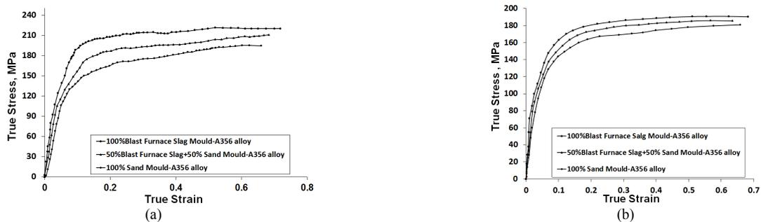
Figure 10: True Stress – true strain curves: (a) under compression testing for aspect ratio (H/D) =1.0, (b) Under tensile testing.
