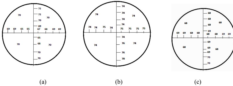
Figure 8: Hardness profiles of A356 aluminium alloy along the cross section of the sample, cast in various moulds of: (a) 100% Silica Sand (b) 100% GBF Slag and (c) Mixture of 50% GBF slag and 50% Silica sand
