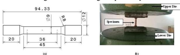
Figure 2: (a) Standard tensile specimen (b) Closer view of the tensile testing.
