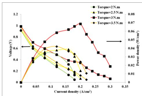
Fig.4 Effect of torque on each bolt on the performance of the fuel cell
