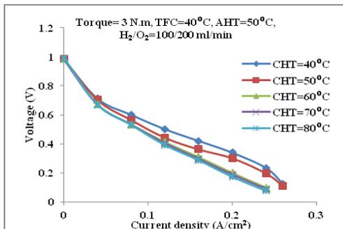
Fig.6. Polarization curves for different CHTs
