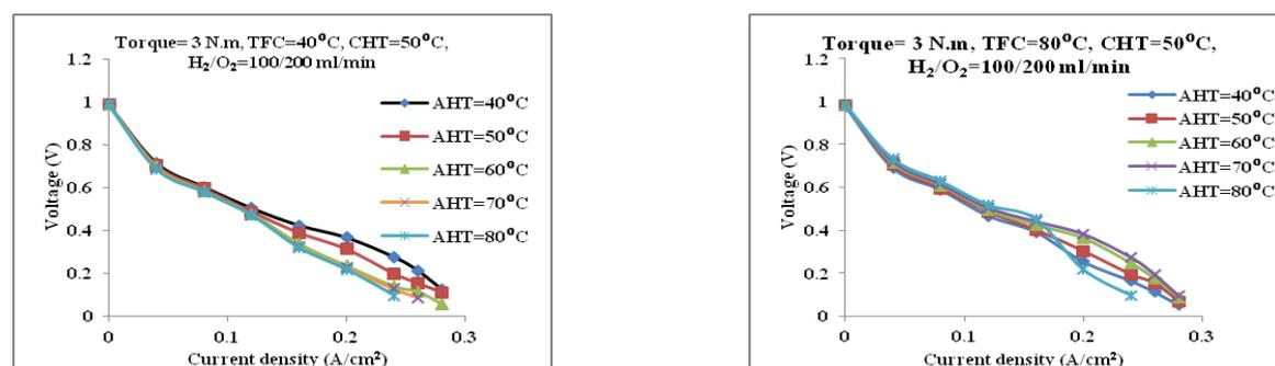
Fig.5. Polarization curves for different AHTs; (a) TFC=40°C; (b) TFC=80°C;
