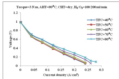
Fig.7. Polarization curves for different TFCs
