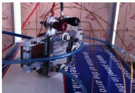
Fig. 1 Transparent single PEM fuel cell
