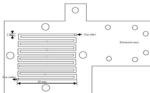
Fig.2 Schematic of titanium gas distributor plate
