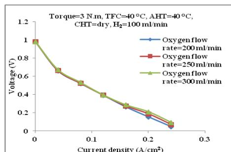
Fig.8. Polarization curves for different oxygen flow rates
