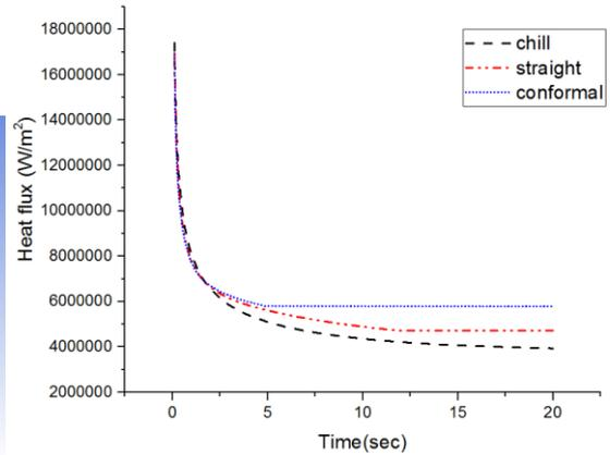
Fig 11. Comparison of Heat flux for different cooling methods
