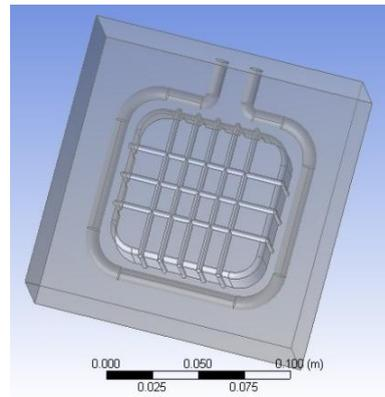
Fig 6. Conformal cooling channel in the mould
