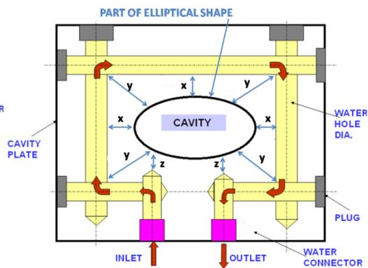
Fig 4. Straight channel for contoured part with uneven cooling
