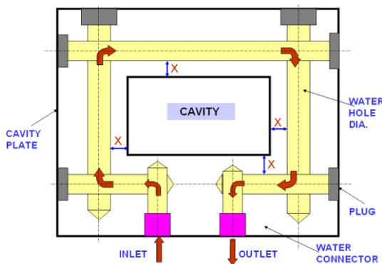
Fig 3. Straight cooling channel equidistant from part [9]
