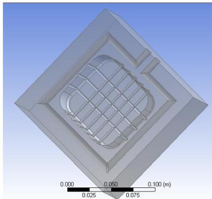
Fig 5. Straight drilled cooling channel
