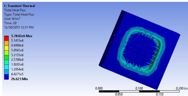
Fig 10. Heat flux for conformal cooling channels after 20 sec
