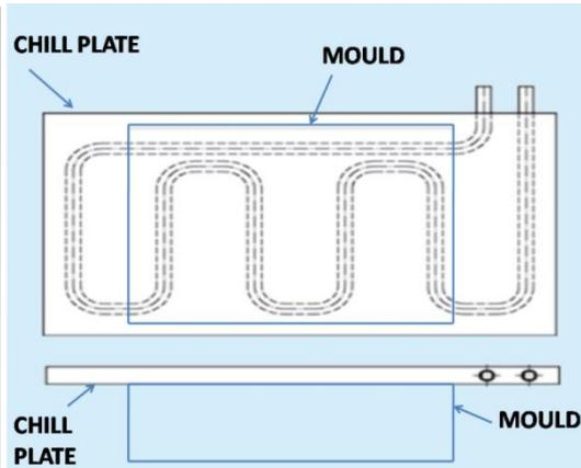
Fig 2. Chill plate attached to the mould for cooling
