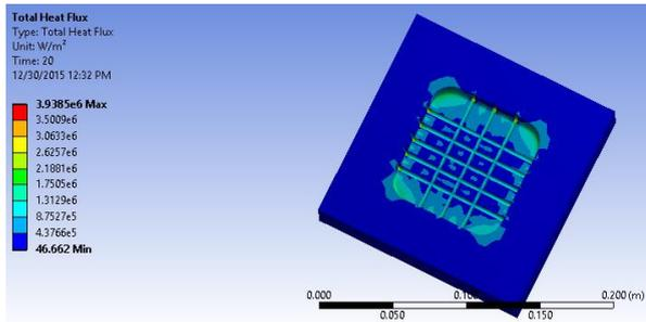
Fig 8. Heat flux after 20 sec when chilled plate at 20°C is attached
