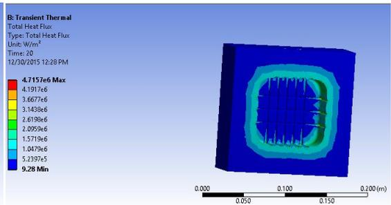
Fig 9. Heat flux for Straight cooling channels after 20 sec
