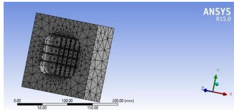
Fig 7. Meshed model in ANSYS
