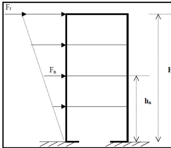
Fig. 1. Vertical repartition of seismic forces [6]
