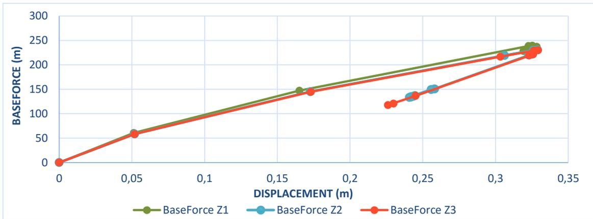
Fig. 3. Pushover curve of unreinforced structure for three zone
