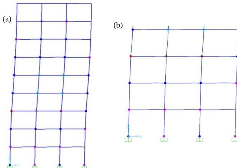
Fig. 2. (a) Plastic hinge formation in the unreinforced structure for zone 3; (b) Zoom on the lower of the unreinforced structure for zone 3.
