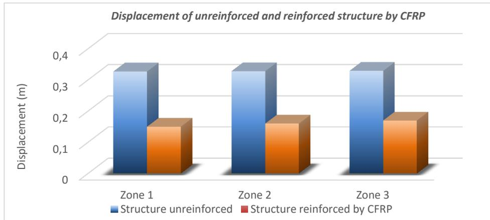
Fig. 5. Comparison of displacement for the two structures
