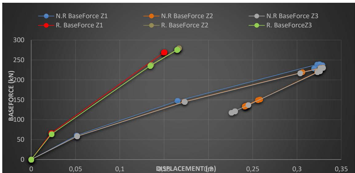
Fig. 4. Pushover Curves of the two structures in three three zones
