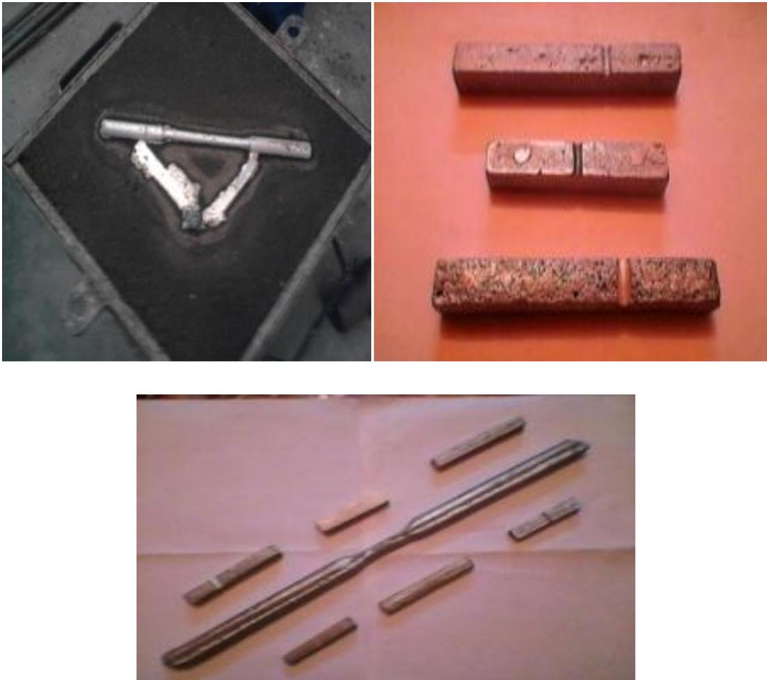
Fig.2- Sample of impact and fatigue test( Ajay singh, et. al, 2013)
