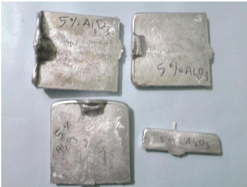
Fig.4 - Sample of aluminium based metal matrix composite
