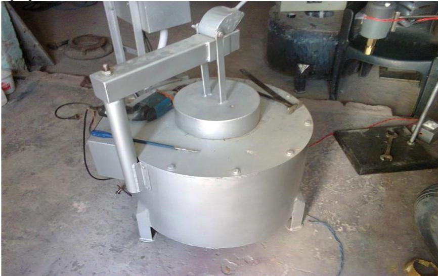
Fig. 3 – Stir casting set up
