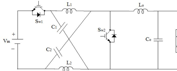
Fig. 3. Impedance source DC-DC converter.
