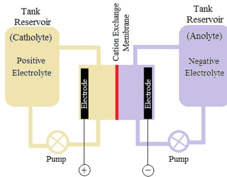
Fig. 1. Configuration of VRF battery.
