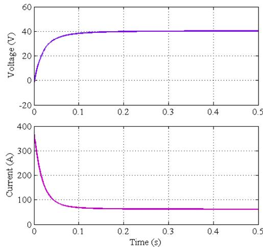
Fig. 4. Voltage and current waveforms of VRFB.
