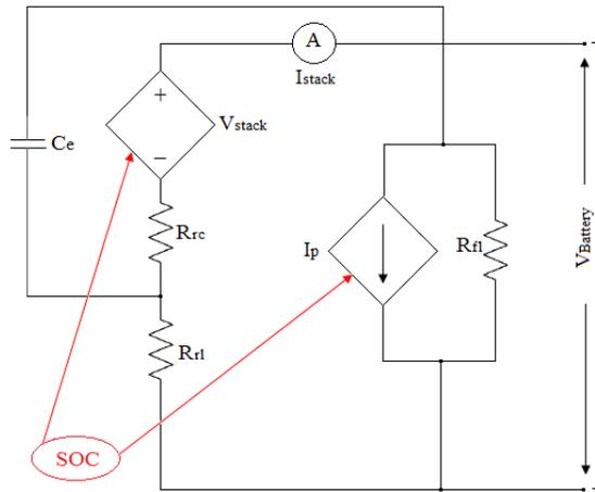
Fig. 2. Equivalent circuit of VRF battery.
