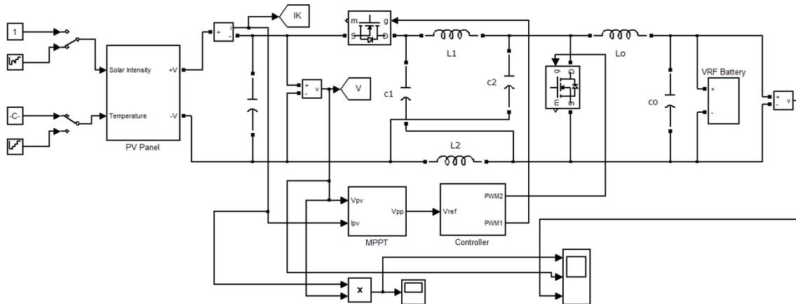
Fig. 5. MATLAB model of PV panel-VRFB system.
