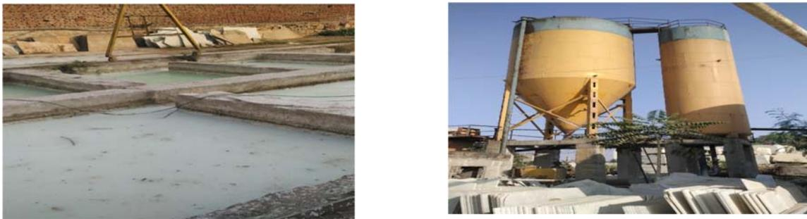
Fig. 1. (a) Sedimentation pits, (b) Sedimentation and filtration towers
