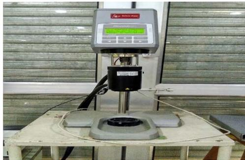
Fig.5 Rheometer setup
